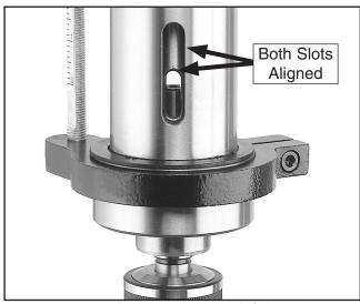
Figure 31. Inner and outer drift-key slots aligned.
